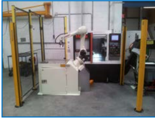
Kawasaki FS006L with Raster loading a Mazak Quickturn Smart
