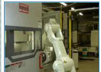
Kawasaki FS010L with Vision loading a Quasar MV154PL
