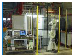
Kawasaki FS006L with Vision loading a Haas Minimill
