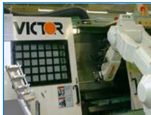
Kawasaki FS020N with Vision loading a Victor
