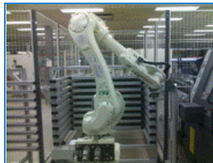
Kawasaki RS020N with magazine loading a Nakamura-Tome
