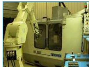
Kawasaki FS030N with Vision loading a Micron VCE1000
