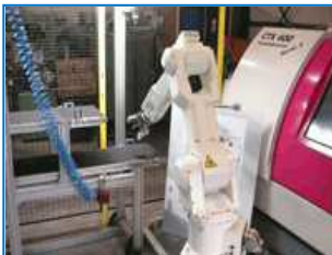
Kawasaki FS010E with Vision and Bin-Picking loading Gildemeister
