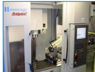
Kawasaki FS010E with Vision loading a Bridgeport VMC610 X3
