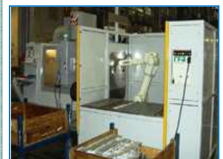
Kawasaki FS006L with raster magazine loading a Hartford VMC560
