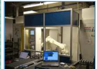
Kawasaki FS006 with Vision loading 2 Fanuc Robotdrills
