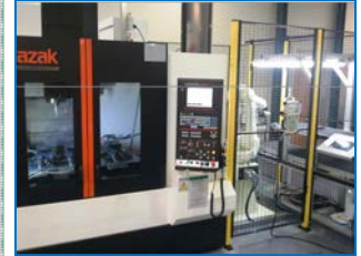
Kawasaki RS010N with Vision loading a Mazak VCS-530C
