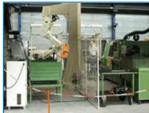
Kawasaki FS045N with Vision loading 2 Mori Seiki
