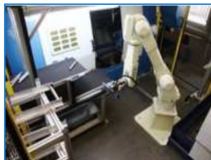
Kawasaki FS010L with Vision loading a Femco
