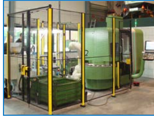
Kawasaki RS020N with Vision and Bin-Picking loading DMG CTV160
