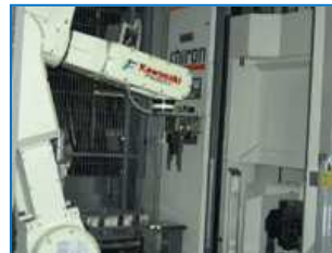
Kawasaki FS020N with Cognex Vision loading a Chiron
