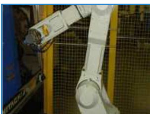
Kawasaki FS020N with raster magazine loading a Hitachi
