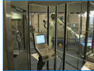
Kawasaki ZX130L with Vision loading a DMG 50EVO
