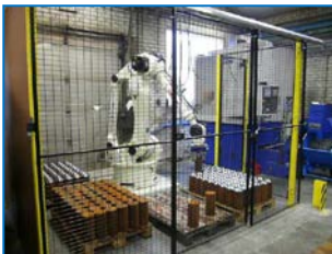
Kawasaki ZX165U picks work pieces from a pallet for a Doosan Puma
