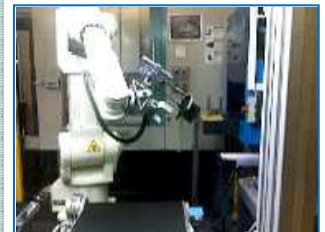
Kawasaki FS006 with Vision loading a Brother TC32B
